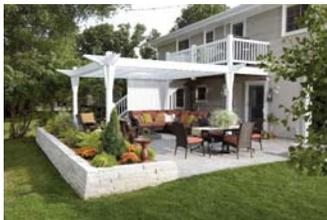
The Druskin's new outdoor space is a marriage of patio design and landscape architecture. In order to create the room-like features that Kristi wanted, we constructed a "floor" of permeable stone pavers and then added "walls" and a "ceiling" using stone planters filled with perennials and a pergola.
